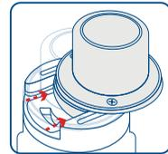
Push in the direction of the arrow, to slide open top cap
